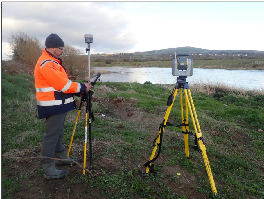
Plate 2: Working shot of DGPS/Total Station set-up.
